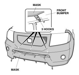
Route the four upper straps at the lower grille area into the front bumper, and attach the loops on the four upper straps to the hooks on the bottom of the mask.
