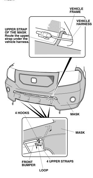
10. Attach the two plastic hooks to the bottom inside edge of the front bumper as shown.
