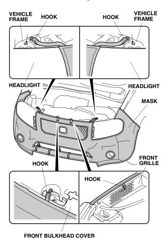
7. On each side, insert the two tabs between the front grille and the headlight.
